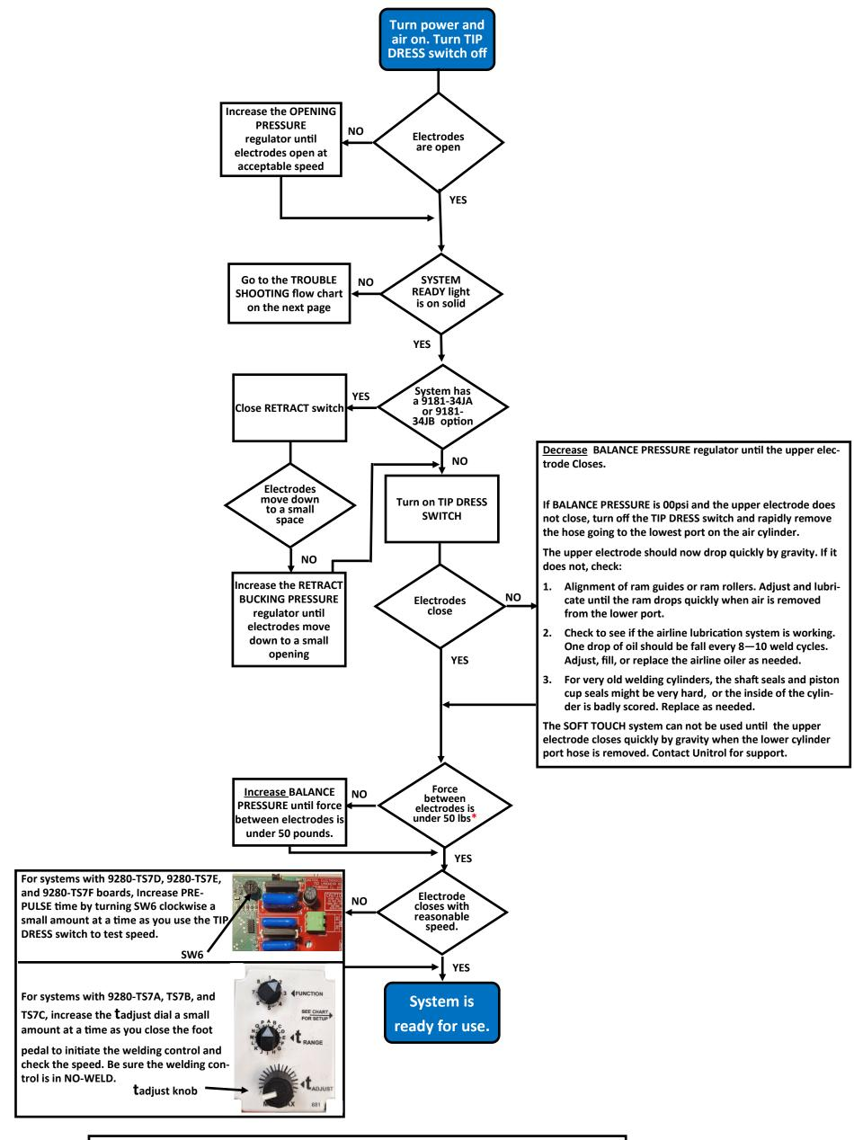
\* If you don't have a tip force measuring instrument, place a wooden office pencil between the electrodes and turn on the TIP DRESS switch. Set the force so that the electrode indents 1/16" or less.
